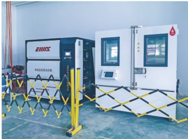
储能变流器防孤岛负载箱 PCS test anti-islanding Load bank
