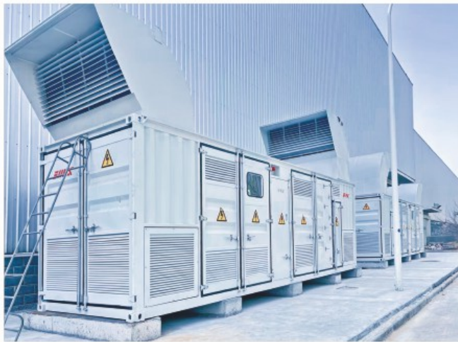
某央企动力测试项目10.5KV-3300KW-RLC负载箱 A central enterprise power test project 10.5KV-3300KW-RLC Load bank
